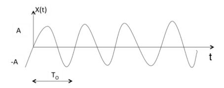
The above signal will repeat for every time interval  $T_0$  hence it is periodic with period  $T_0$ .
