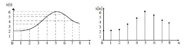
In the above example, the sampling time interval was T=1sec, which means samples are taken after every 1 sec to form the discrete time signal.
