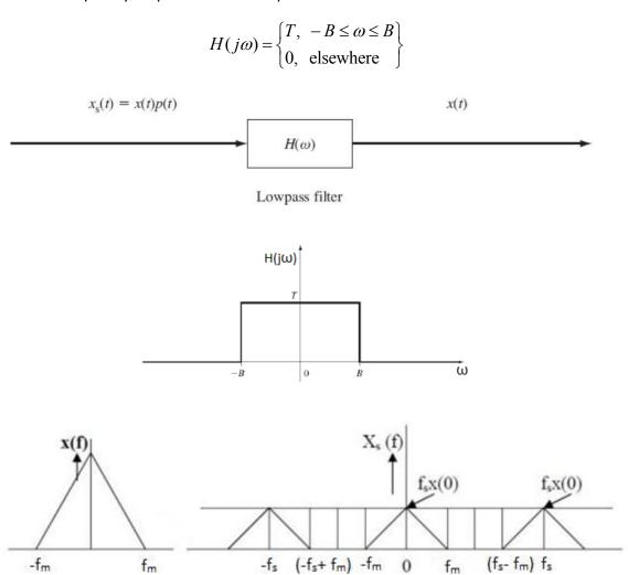
Reconstruction process is possible only if the shaded parts do not overlap. This means that  $f_s$  must be greater that twice  $f_{\it m}$ .
