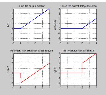
The correct one is exactly like the original function but shifted.
