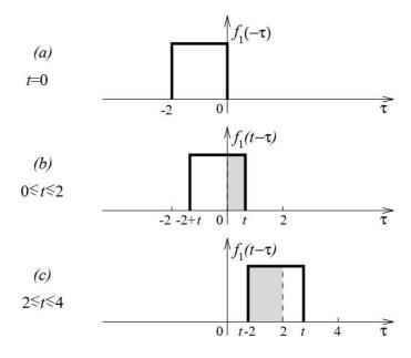
The convolution integral in these two intervals, evaluated according to information given in Figures b and c, is respectively given by
