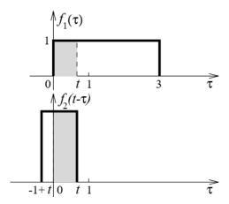
It can be seen from Figure that in the interval from zero to the signals overlap, hence their product is different from zero in this interval, which implies that the convolution integral is given by
