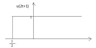
(always do scaling first, then shifting. In this case since it's a unit step function, there is no effect on scaling. ) ie  $u(2(t+\frac{1}{2}))$
