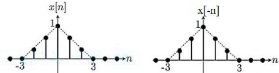
Example: As shown in the following diagram, rectangle function x(t) = x(-t) so it is even function.
