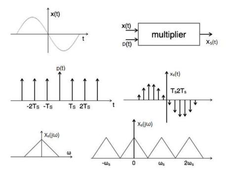
Sampling of input signal x(t) can be obtained by multiplying x(t) with an impulse train p(t) of period  $T_s$ . The output of multiplier is a discrete signal called sampled signal which is represented with  $x_s(t)$  in the following diagrams:
