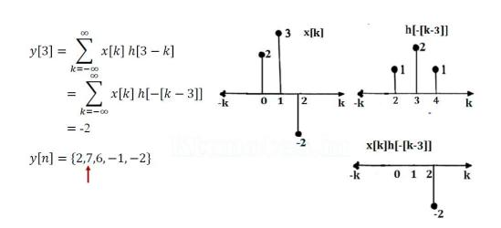
Number of samples in y[n] or length of linear convolution=L(length of x[n]) +M(length of h[n])-1 = 3+3-1=5
