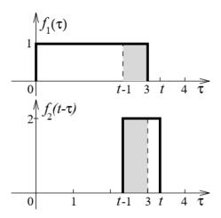
$$f_1(t)*f_2(t) = \int\limits_{t-1}^3 1 imes 2d au = 8-2t, \quad 3 \le t \le 4$$
