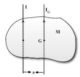
Let  $I_G$  be the moment of inertia of a body of mass M about through the center of gravity and I be the moment of inertia about a parallel axis at a distance 'a' from the center of gravity. Then according to parallel axis theorem,
