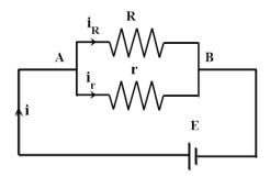
Consider a large resistance R and a small resistance r connected to a source emf as shown in the figure. Let  $i_R$  and  $i_r$  be the currents flowing through them. If i is the main current entering the junction A,
