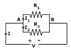
Consider two resistors  $R_1$  and  $R_2$  connected in parallel so that both have the same potential difference V across the points A and B as shown in the figure. At point A the main current I split into two parts -  $I_1$  through  $R_1$  and  $I_2$  through  $R_2$ . Hence,
