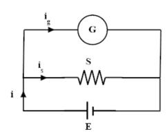
Let G be the resistance of the galvanometer and S is the shunt resistance. If i is the current to be measured,  $i_s$  is the current through the shunt and  $i_g$  is the maximum current which produces full scale deflection in the galvanometer.
