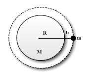
Consider a satellite of mass m revolving around earth of mass M and radius R. Let the satellite be revolving at a height h with an orbital velocity v, above the surface of the earth. The necessary centripetal force for the circular motion is provided by the gravitational force between earth and the satellite.
