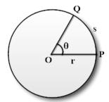
Consider a body moving around the circumference of a circle with center 'O' and radius 'r'. The linear displacement of the body as it travels from P to Q in 't' seconds is 's'.
