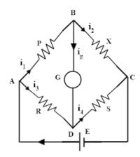
Wheatstone's bridge is a network of four resistances commonly used for the measurement of resistance. Three resistance boxes P, R and S and an unknown resistance X are connected as shown in figure. A cell of emf E is connected between A and C and a galvanometer between B and D. Let the resistance of the galvanometer be G and the current through it be  $i_g$ . The currents in various branches are as shown in figure. Applying junction rule at the junctions B and D,
