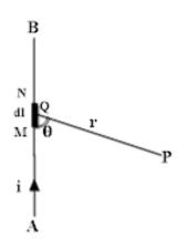
Biot-Savart law help us to determine the magnetic field intensity at a point due to a small current carrying element of the conductor. Let AB represents a conductor through which a current i flows. MN is a very small segment of length dl of the conductor. P is a point at a distance r from the mid point Q of the segment.  $\theta$  is angle between dl and r. Biot-Savart law states that the magnetic field dB produced by an elementary length dl of a current carrying conductor at a point P is
