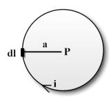
Consider a single turn of a circular coil of radius 'a' carrying a current i. From Biot-Savart law the magnetic field dB at the centre of the coil due to an elementary length dl is
