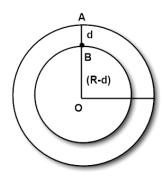
Consider a point B at a depth d below the surface of the earth as shown in the figure. Since the gravitational force due to the shell of earth of thickness d at any point inside the shell is zero, the acceleration due to gravity  $g_d$  at the depth d is obtained by replacing R with (R-d) in equation (2). Thus,
