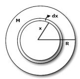
Let M be the mass and R be radius of the disc. the disc can be imagine to be made up of a large number of rings of very small width and gradually increasing radii fro zero to R. Consider a ring of radius x and width dx.
