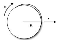
Consider a disc of radius R and mass M. Let the disc be rolling on a horizontal surface without slipping. Rolling motion of the disc is a combination of a translational motion of the center of mass of the disc with velocity v and a circular motion with angular velocity  $\omega$ . Hence the disc has two types of kinetic energies - translational and rotational kinetic energies.
