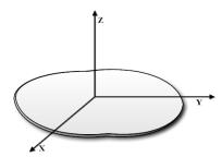
Consider a plane lamina lies in XY plane and Z-axis is perpendicular to the plane of the lamina. Let  $I_X$ ,  $I_Y$  and  $I_Z$  are the moment of inertia of the plane lamina about X,Y and Z axes respectively. Then according to perpendicular axis theorem,
