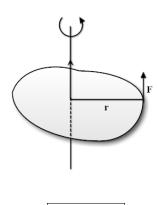
Torque is the rotational equivalent of force and moment of inertia is the rotational equivalent of mass. Therefore comparing equation F = ma, the equation for torque is given by,
