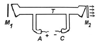
Helium-Neon laser is gas laser. The essential parts of He-Ne laser are shown in the figure. The working substance of this laser is a mixture of helium and neon in the ratio 10:1. The gas mixture is placed in a long discharge tube, typically 50 cm long and 0.5 cm diameter. The pressure inside the tube is nearly 1 mm of mercury. The anode A and cathode C are attached to the side
