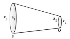
Consider a portion of a pipe PQ of cross sections  $a_1$  and  $a_2$  at the points P and Q respectively. If  $v_1$  and  $v_2$  are the velocities of the liquid crossing the areas  $a_1$  and  $a_2$ , then according to equation of continuity:
