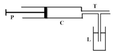
The figure shows the essential parts of an atomiser. C is a cylindrical barrel which terminates in a small tube T. T is connected to a vessel L containing the liquid to be sprayed. When air in the barrel is pushed by the piston P, the speed of the air increases considerable in tube T. According to Bernoulli's principle, this causes a reduction in pressure. As a result, the liquid in the vessel rushes up and mix with high speed air to form a fine spray.
