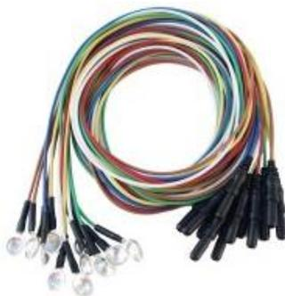
The most commonly electrodes for measuring EEG are the electrodes with chloride silver discs of size 6 to 8 mm diameters. Contact with the scalp is made via an electrolytic paste through a washer of soft felt. They have ac resistance varying from 3 to 20K $\Omega$ .
