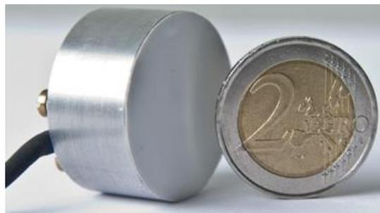
Capacitive type biomedical electrodes have also been used for EMG recordings from the surface of the skin. The anodized aluminium electrodes were not found suitable on a long term
